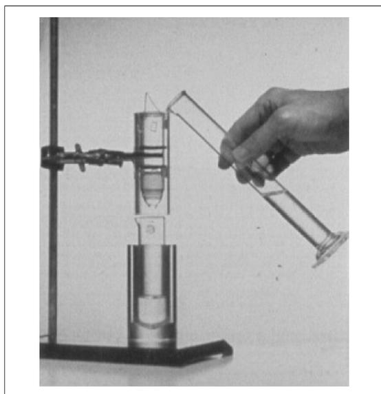
**Figure 1. The Original Mo-99/Tc-99m Generator (Shown Without Lead Shielding)**
