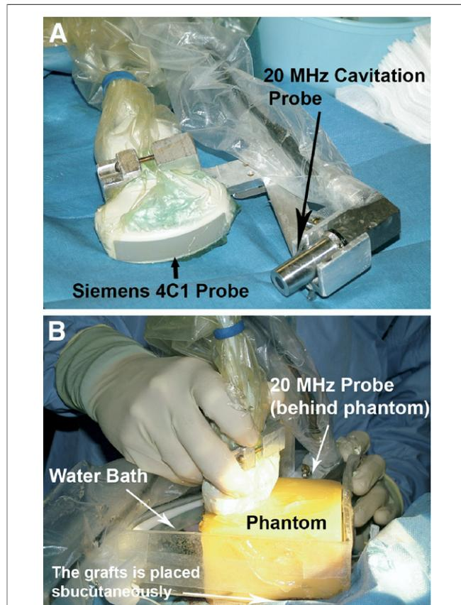
**Figure 1. The Set-Up of the 20-MHz Listening Device**
