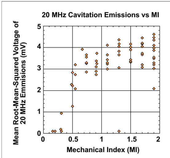
**Figure 4. Cavitation Emissions at Different Mechanical Indexes**
